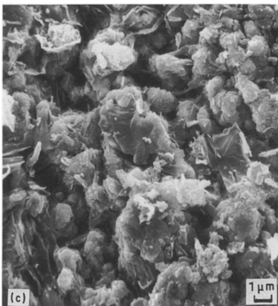
Figure 16 Scanning electron micrographs of an EG coating after holding for 16 h at (a) 100 °C, (b) 200 °C, (c) 300 °C.
